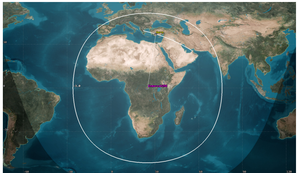
Figure 4. Simulation of the wanted Inmarsat Aero link (space-to-Earth) in the L-band.
