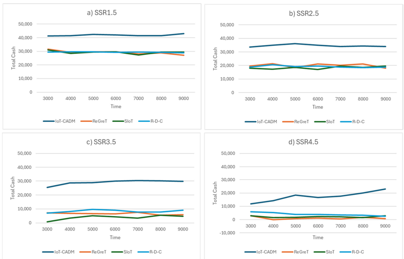
Figure 10. Cash utility for a dishonest environment (0–75%) for (a) 0% dishonest agents, (b) 25% dishonest agents, (c) 50% dishonest agents and (d) 75% dishonest agents.
