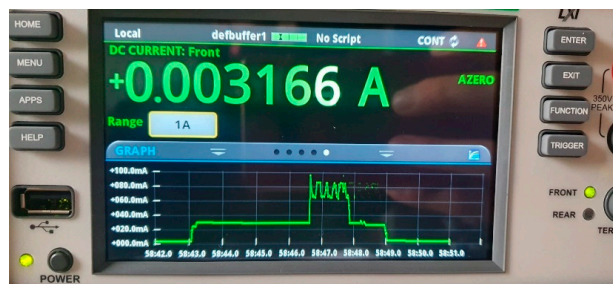
Figure 11. Node’s current consumption in deep sleep mode.
