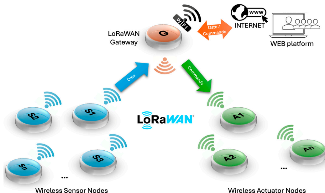
Figure 1. The architecture of the proposed Agri-DSS.
