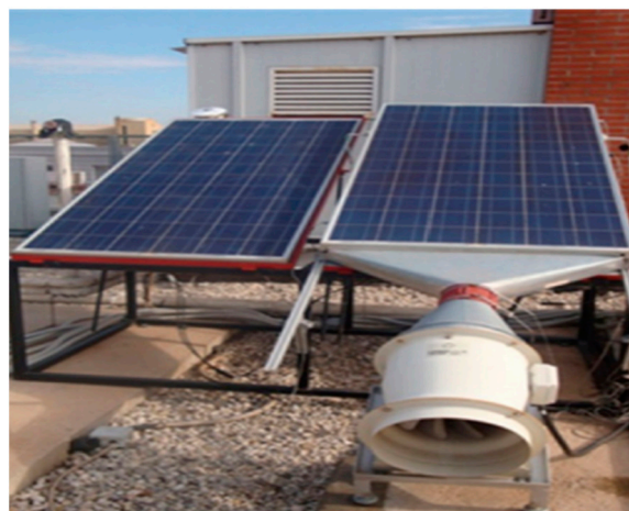
Figure 6. Air-based cooling technique.
