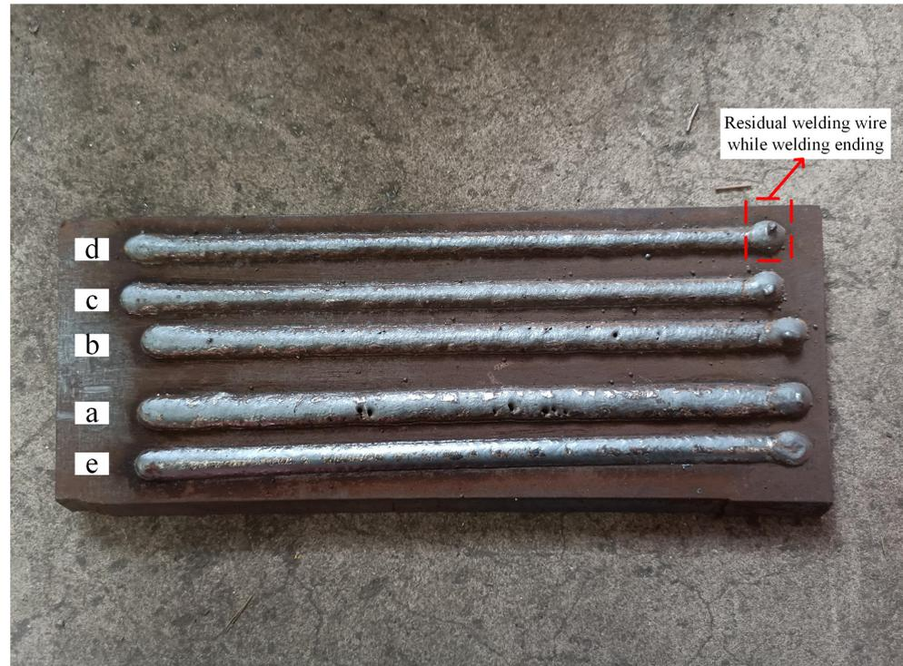
**Figure 8.** Welding experiment results. The application of the proposed vibration suppression method results in the enhanced stability of welding formation quality.
