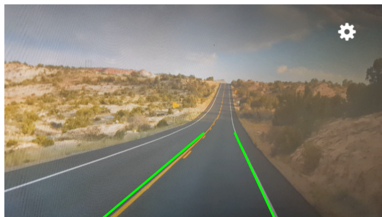
Figure 23. Lane detection on a curved road made by the mobile-phone app.
