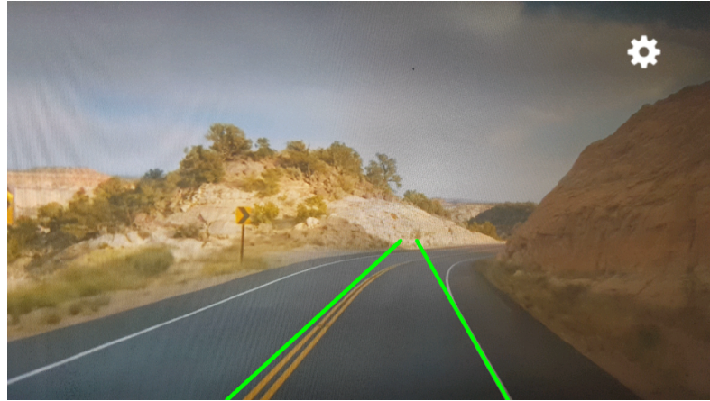
Figure 24. Lane detection on a straight road made by the mobile-phone app.
