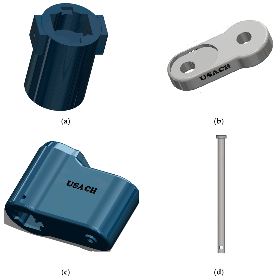
Figure 3. SCARA robot components: (a) base; (b) first arm; (c) second arm; (d) shaft.
