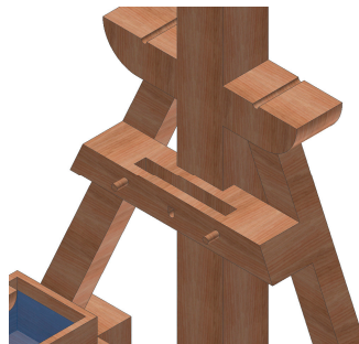
Figure 7. Detail of the base for the shuttle and supports for the horizontal cylinders.
