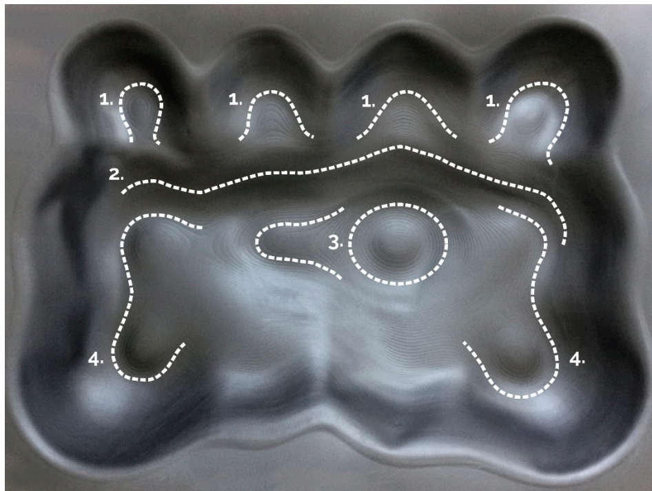
Figure 5. Types of erroneous features in the first mold: (1) Highland, (2) Brink, (3) Hillock with surrounding depression, and (4) Bay.
