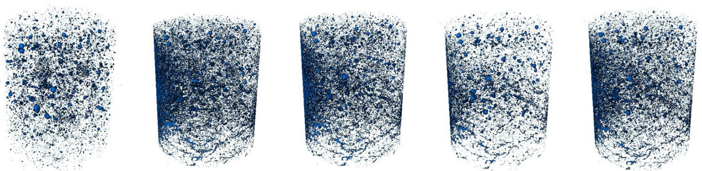
Figure 8. Example of pore evolution over time. From left to right: 1, 2, 3, 4, and 7 days age.
