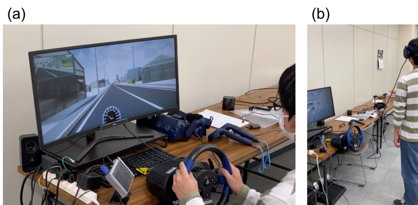
Figure 13. Tsunami evacuation training simulator system: (a) simulation of evacuation by car and (b) simulation of evacuation on foot.
