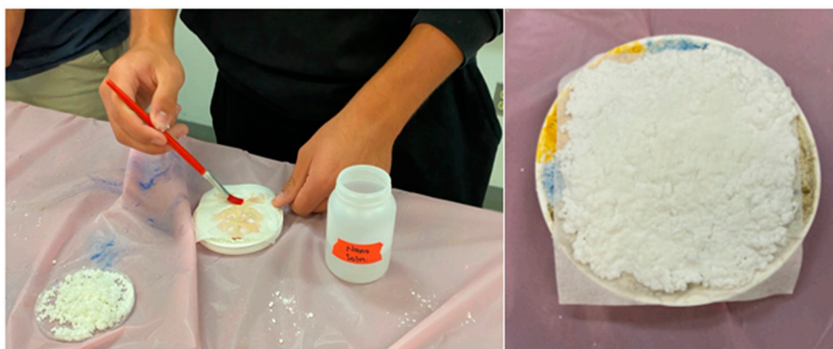
Figure 8. Day 6: the students apply \text{Ca(OH)}_2 through Japanese rice paper and damp Arbocel onto their fresco to complete the conservation process.
