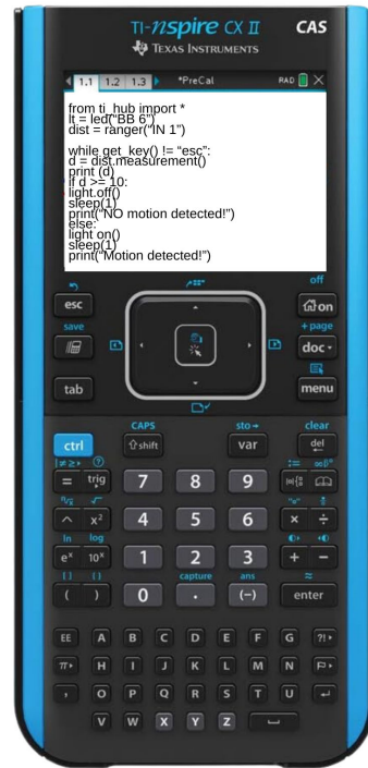
Figure 3. Texas Instruments Python coding for detecting distance.
