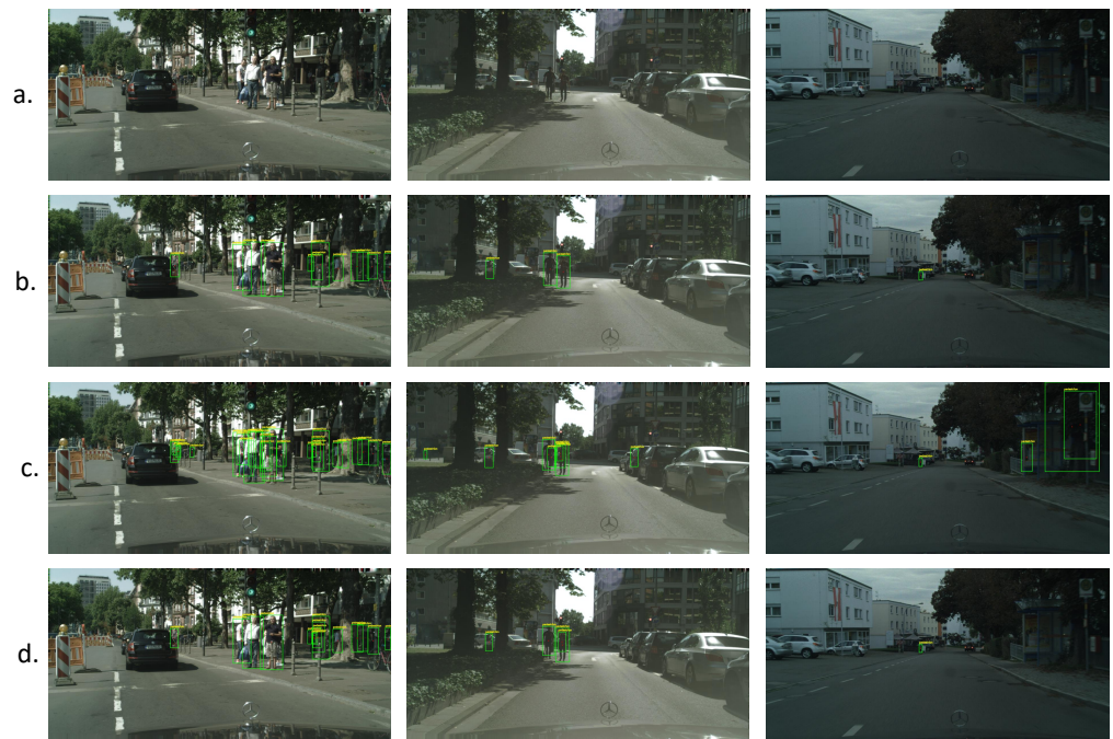
Figure 6. Visualization results of CCFNet and CSP do not limit the visibility of pedestrian objects. (a) Input the original image for the CityPersons dataset; (b) is the ground truth corresponding to (a); (c) is the visualization result of CSP; (d) is the visualization result of CCFNet.
