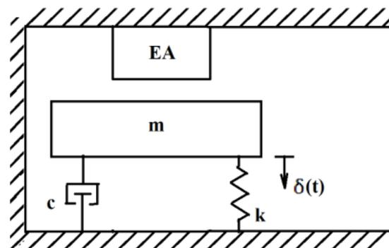
Figure 1. Sketch of damped, forced Hertzian oscillator with an asymmetric EA.
