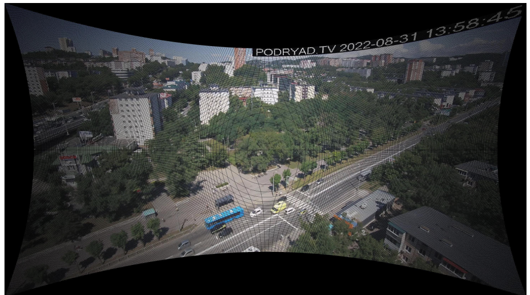
Figure 10. The image \Phi after compensation of radial distortion; Example 2, image \hat{\Phi} = \Theta(\Phi) without postprocessing.
