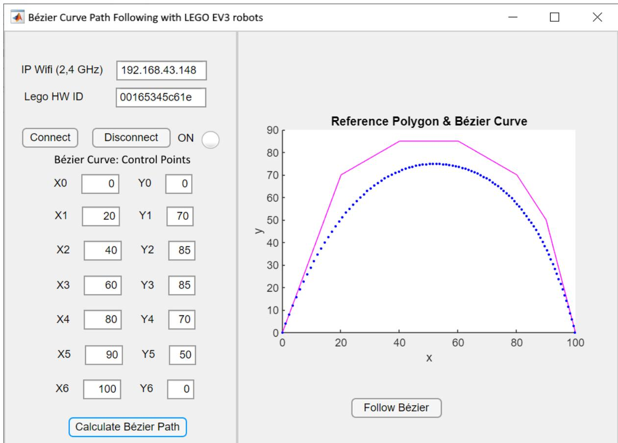
Figure 4. Matlab Application for the LEGO EV3 robot control.
