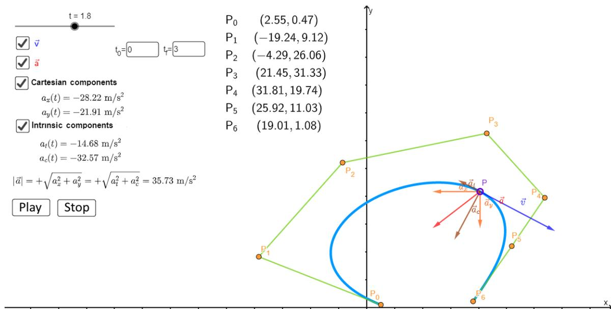
Figure 2. A particular example of robot path design using Bézier covers with the GeoGebra applet.
