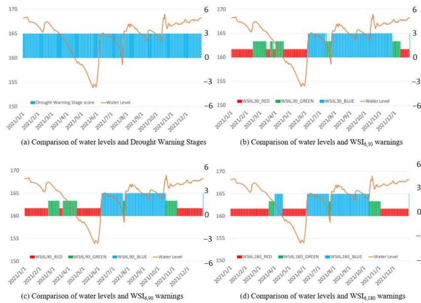
Figure 12. Comparison of the Water Conservancy Drought Warning Stage with the WSI_{6,j} proposed in this study.
