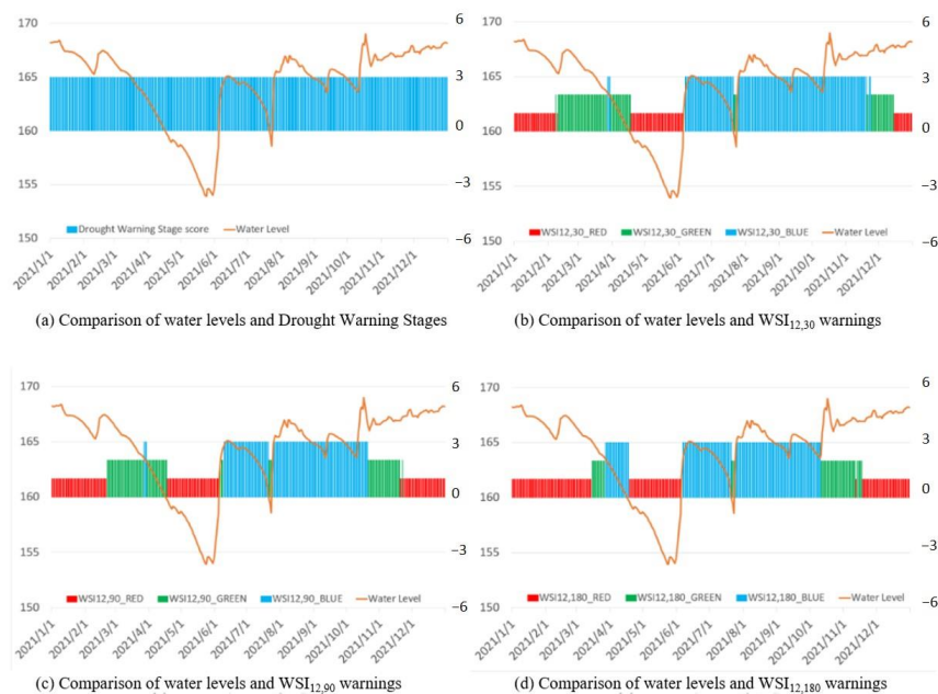
Figure 13. Comparison of the Water Conservancy Drought Warning Stage with the WSI_{12,j} proposed in this study.
