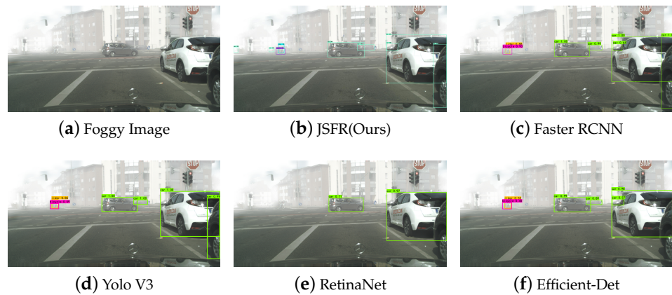
Figure 6. Test results of JSFU and object detection methods including Faster RCNN , Yolo V3 , RetinaNet and Efficient-Det on Foggy Cityscapes with sparse fog (electronic zoom-in recommended).
