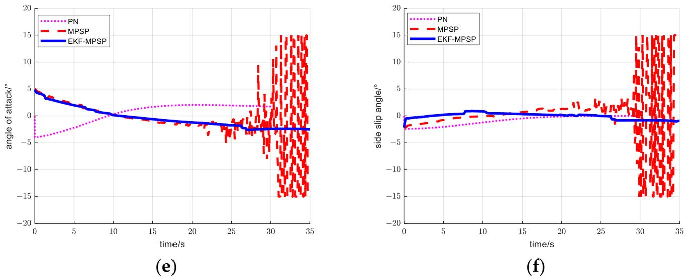
**Figure 3.** Comparative simulation results of three methods: (a) three-dimensional trajectory; (b) missile velocity profiles; (c) path angle profiles; (d) azimuth angle profiles; (e) angle-of-attack profiles; and (f) side slip angle profiles.
