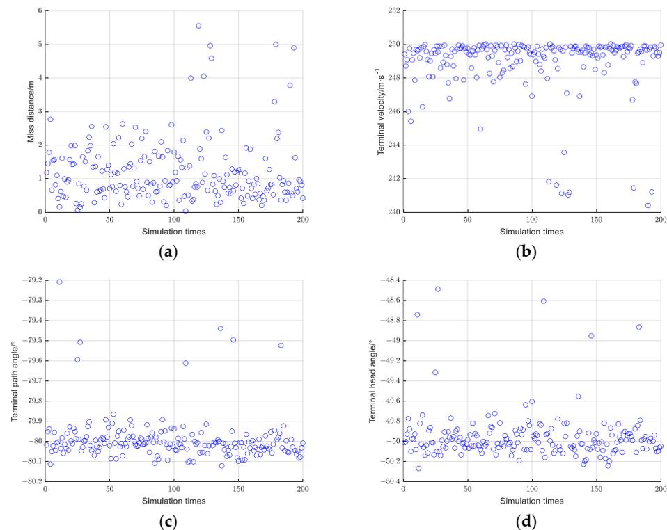
**Figure 5.** Monte Carlo simulation results: (a) terminal miss distance; (b) terminal velocity; (c) path angle profiles; and (d) azimuth angle profiles.
