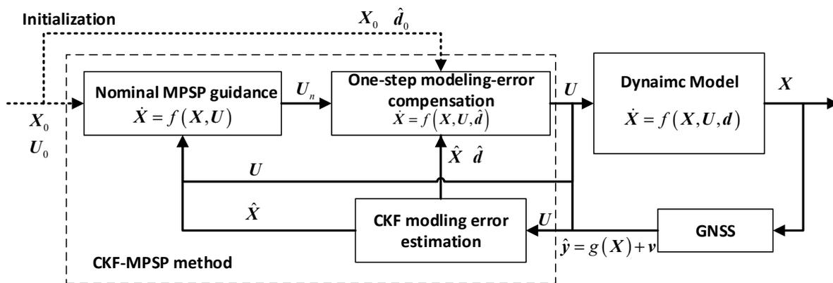
Figure 2. CKF-MPSP guidance method schematic.
