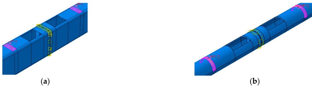
Figure 14. Loading areas for: (a) RHS; (b) CHS.
