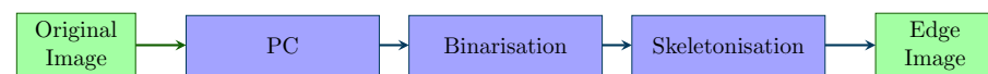
Figure 5. Block diagram of the proposed method for edge detection using phase congruency.
