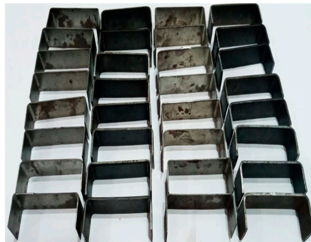
Figure 7. Folded parts after experimental folding tests.
