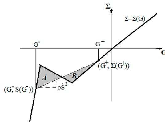
Figure 2. The stress–strain diagram with jumping of strains.
