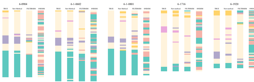
Figure 17. Comparison of borehole results simulated by three methods.
