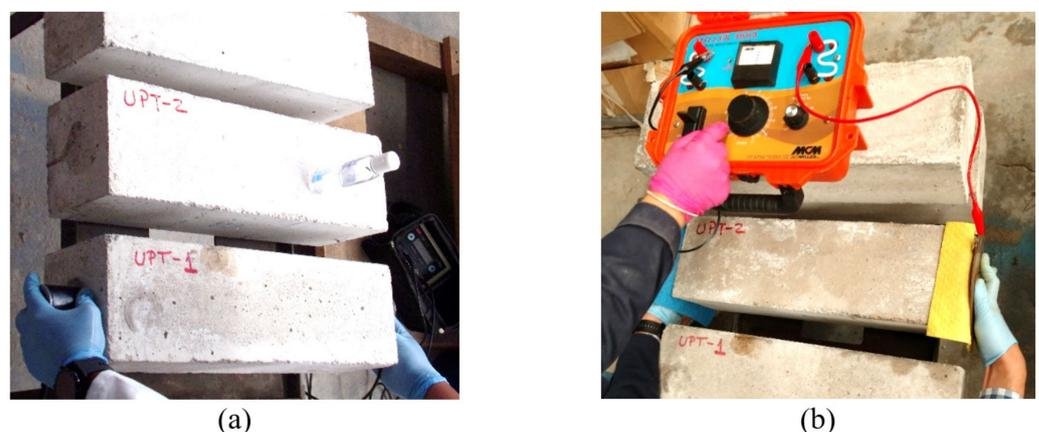
**Figure 9.** Pictures from tests for some specimens: (a) UPVT and (b) Resistivity tests.
