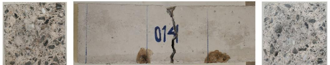
**Figure 14.** Concrete beam No. 14 fractured after the bending test, showing the lower view and the fractured faces at the ends (cross-sectional areas).
