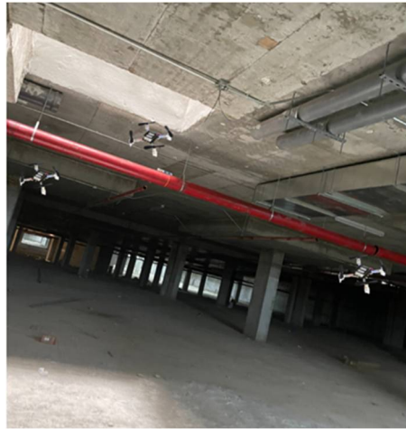
Figure 1. An operational scenario of a multi-UAV inspection mission.
