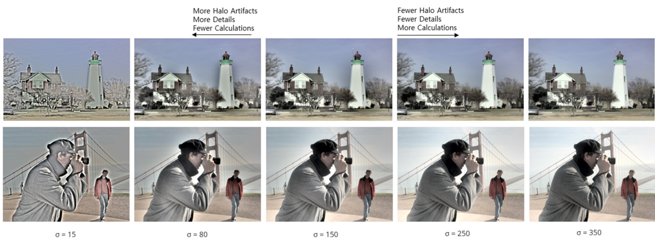
Figure 1. Comparisons of the single-scale Retinex method with various standard deviation ( \sigma ) values.
