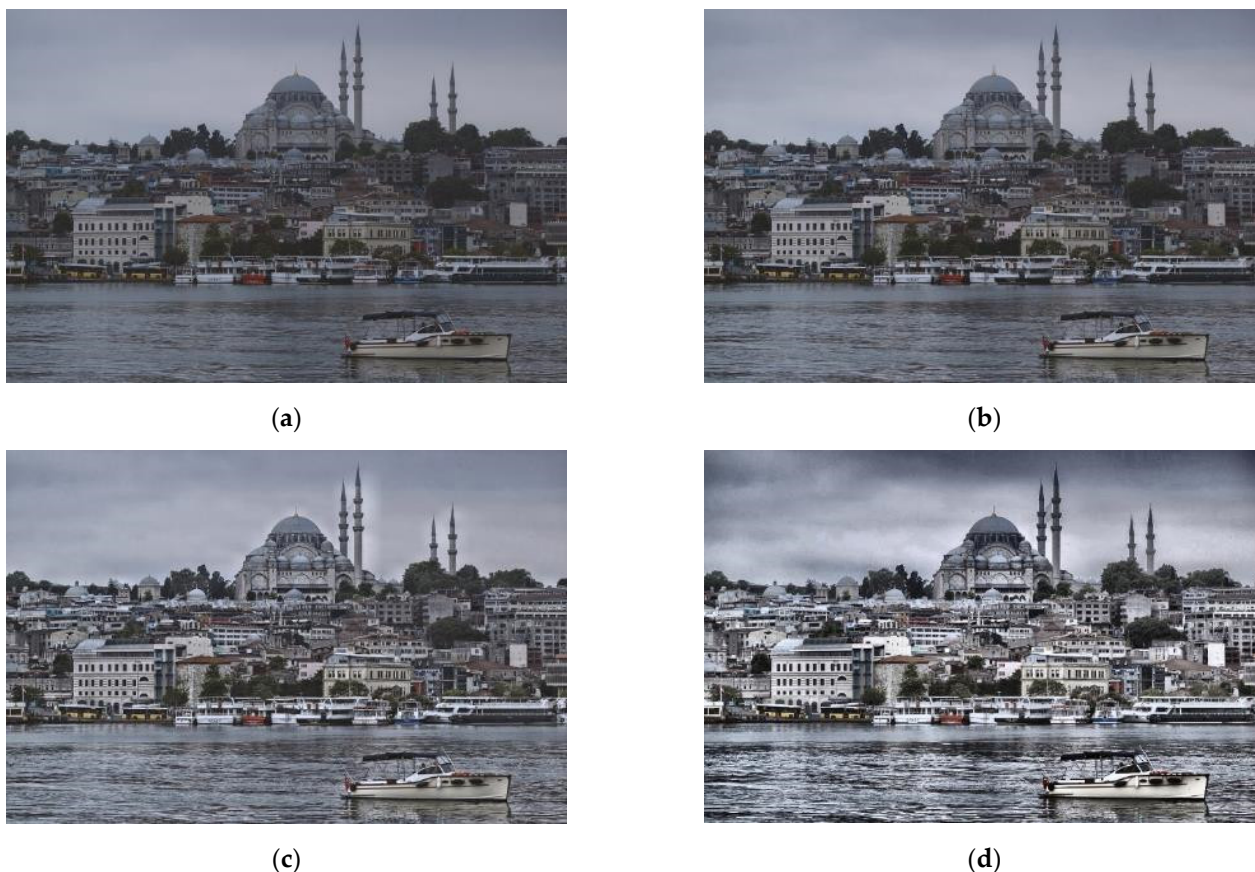
Figure 2. Problems with incorrect parameter values for a single-scale CLAHE: (a) Original image, (b) low-enhanced image with low parameter values, (c) increased halo artifacts due to the high TileSize, and (d) increased noise due to the high ClipLimit.
