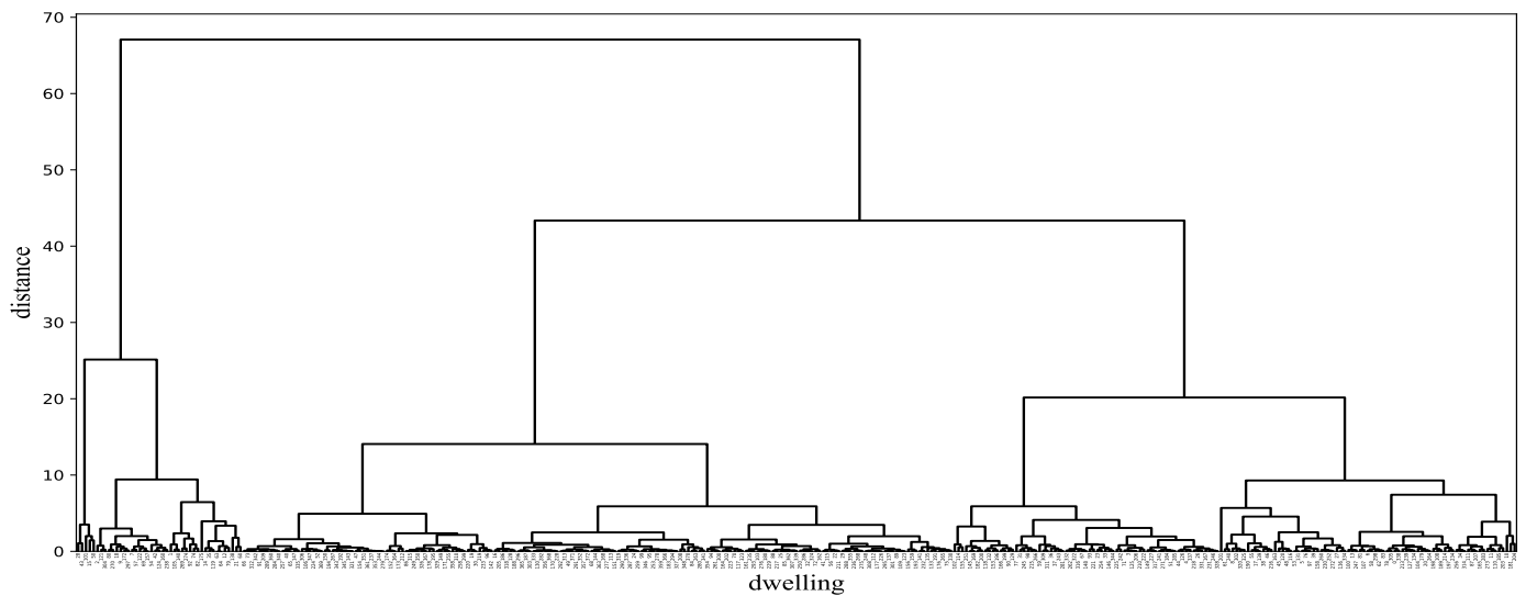
Figure 15. Dendrogram of the AHC process with the Ward linkage method for data of electrical load power consumption in Brazil.
