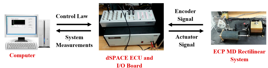
Figure 14. Structure of dSPACE-based digitally controlled ECP MD rectilinear system.
