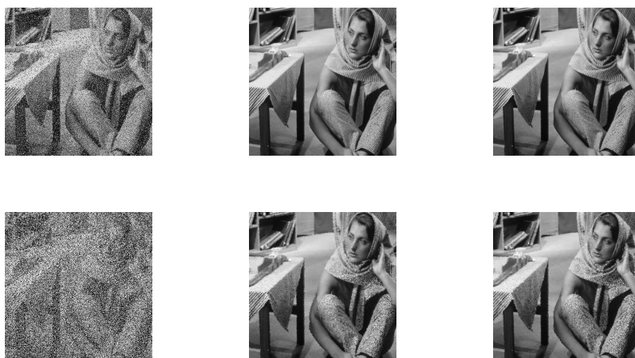
Figure 6. The noisy Barbara image, corrupted by salt-and pepper noise (the first column); the images restored via Algorithm 1 (the second column), and via the MHSCG method (the third column).
