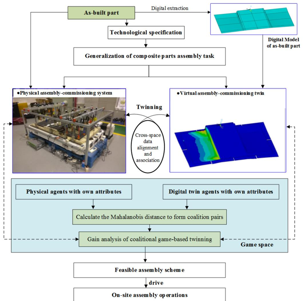
Figure 4. Overall framework of digital-twin-driven assembly process decision making.
