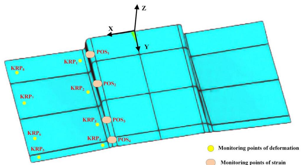
Figure 7. Monitoring points of deformation and strain.
