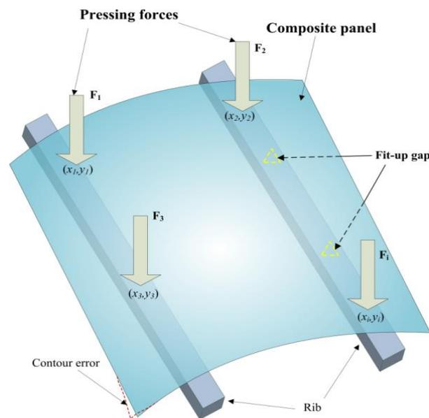
**Figure 3.** Large thin composite skin added to the frame components (stringers and ribs).
