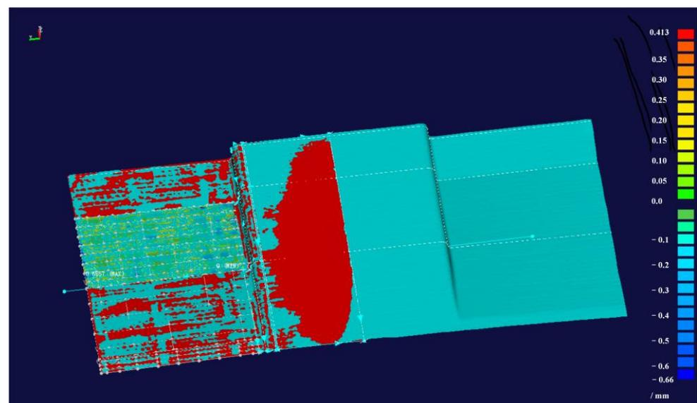
**Figure 6.** Error distribution between 3D point cloud and the abstract model of the as-fabricated composite panel.
