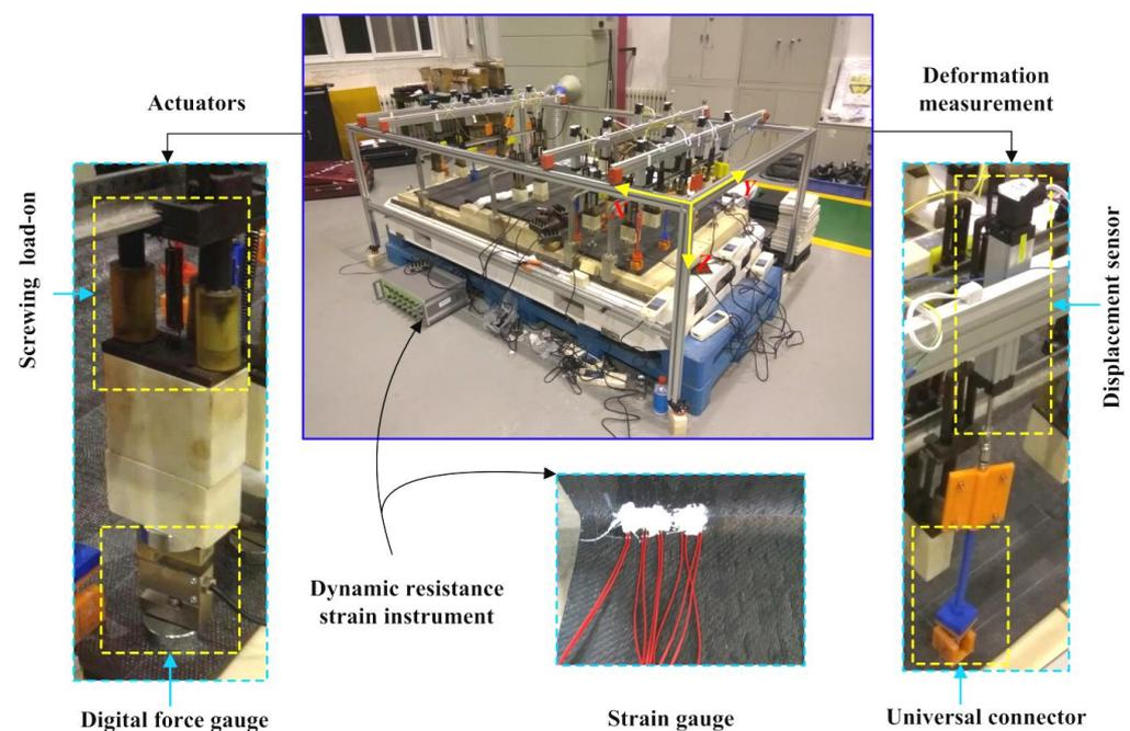
**Figure 5.** Physical assembly-commissioning system.
