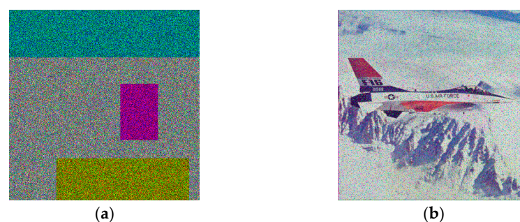
Figure 20. Blocking attack. (a) Picture after channel loss; (b) Decrypted image after the attack.
