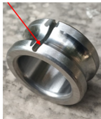
Figure 7. Inner race defect.
