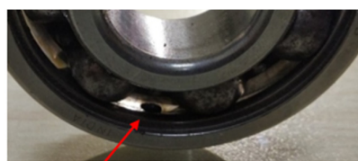
Outer race defect
