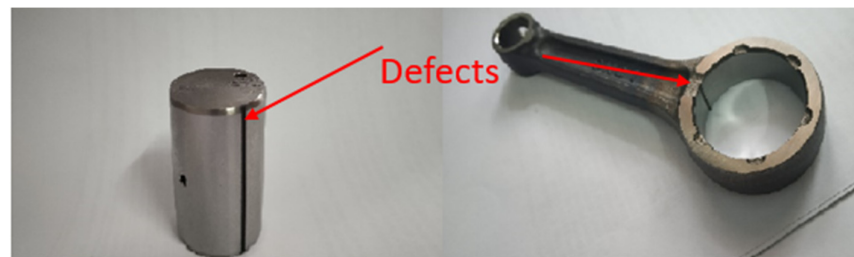
Figure 9. Crank pin and connecting rod defect.
