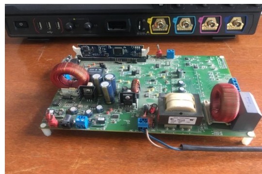
Figure 34. DSP control platform.
