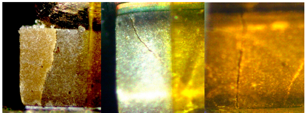
Figure 6. Cracks on the piezoelectric elements of multiple PVSs with out-of-sensitivity.
