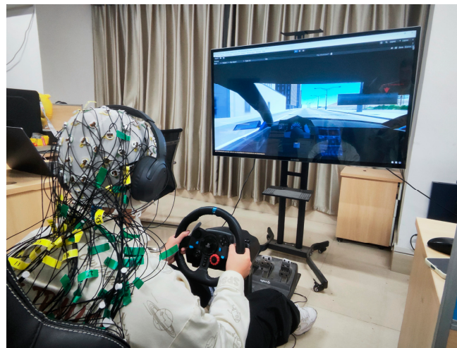
Figure 3. EEG signal test scenario.
