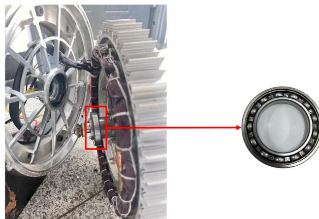
Figure 5. Schematic diagram of the rotor motor to replace the faulty bearing.
