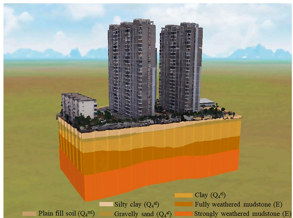
**Figure 14.** Integrated surface building and subsurface engineering geological models.
