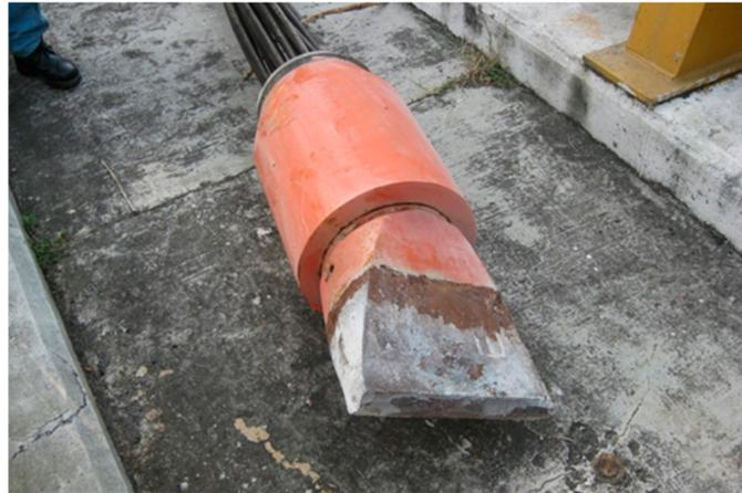
**Figure 5.** Failed anchoring element of cable 1 semi-harp 5 (T1S5).
