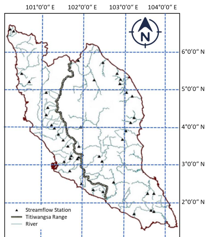
Figure 1. Locations of 41 streamflow stations with 227 rainfall-runoff (P-Q) data pairs used for \lambda derivation. Modified according to [21].
