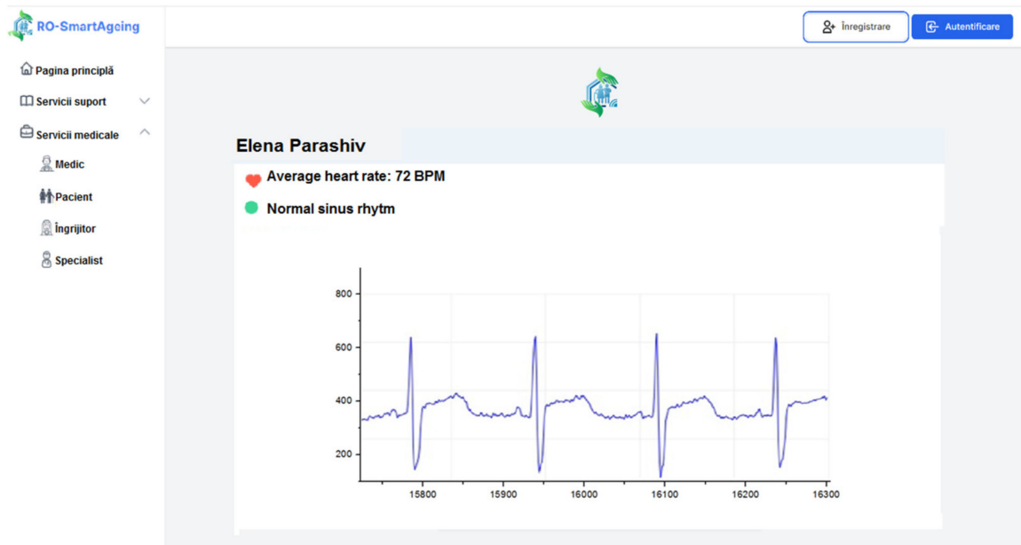
Figure 9. Measured ECG with the Medical Blackbox displayed on the RO-SmartAgeing platform.
