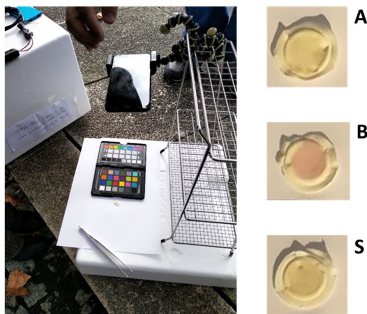
Figure 4. Set-up for in-field screening of SMZ and results from a test sample S (A—negative control, absence of SMZ; B—positive control, SMZ at 25 \mu\text{g L}^{-1} ).
