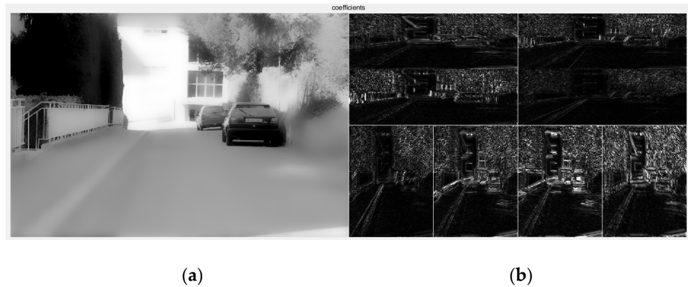
Figure 3. Result of the base and edge images decomposed by contourlet transform: (a) base and (b) edge images (eight directions).
