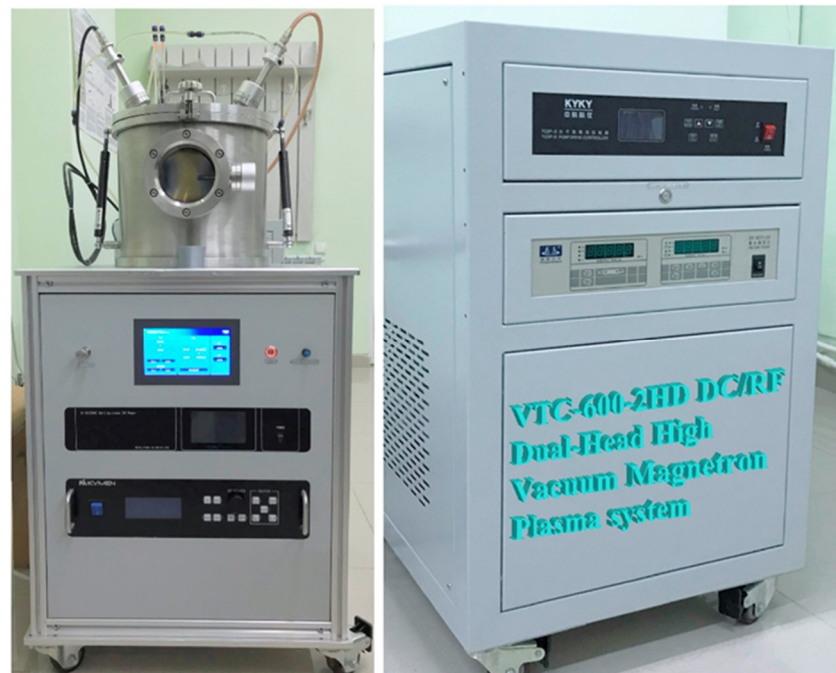
Figure 2. Actual photograph of the VTC-600-2HD DC/RF Dual-Head High Vacuum Magnetron Plasma System.
