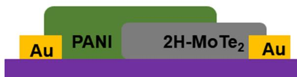
**Figure 1.** Schematic diagram of the layered heterostructured sensor device composed of 2H-MoTe<sub>2</sub> film and PANI film.
