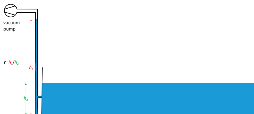
Figure 1. Hydraulic analogy of AGNES. The liquid (in blue) in the large vessel at the right hand side is open to the atmosphere, and its level ( h_2 ) is practically not affected by changes in the amount of liquid in the left hand side tube, where the liquid reaches a higher level ( h_1 ) due to the vacuum pump suction. The gain ( Y ) would be the ratio between the two levels. file:HydraulicAnalogy.pptx.
