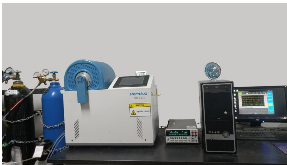
Figure 1. Photograph of the commercial gas sensing system (GRMS-215, Partulab Com., Wuhan, China) used in this study.
