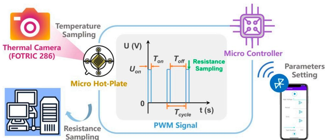
**Figure 1.** The measuring system for MEMS gas sensors.
