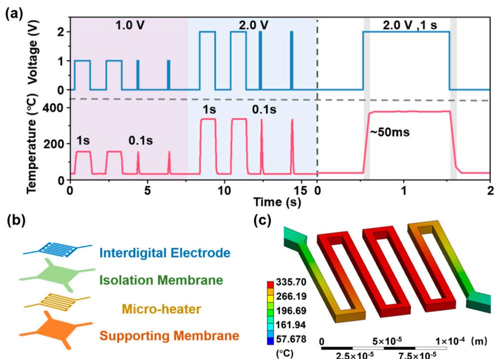
**Figure 2.** (a) The temperature variation in the MHP's surface under different heating voltage. (b) The schematic diagram of the MHP's four-layer structure. (c) The temperature distribution of the MHP by finite element analysis under 2.0 V.
