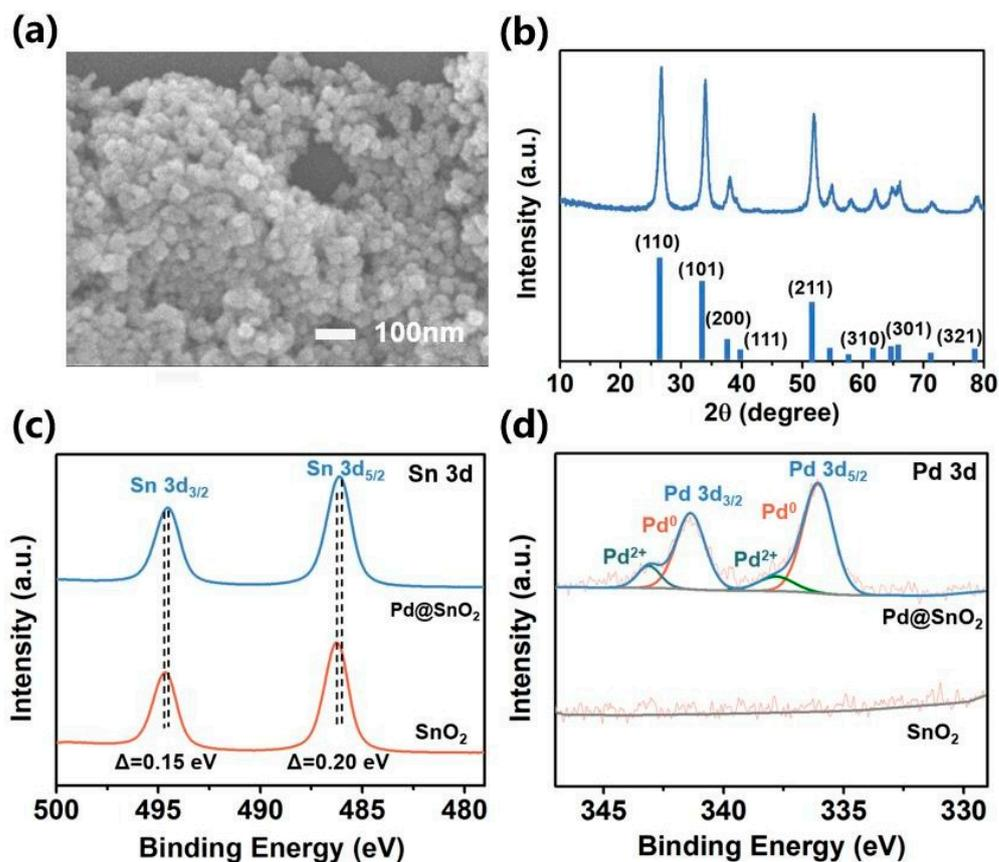
**Figure 5.** (a) SEM image (b) XRD pattern (c) XPS Sn 3d and (d) XPS Pd 3d of the prepared Pd-doped SnO<sub>2</sub> particles.
