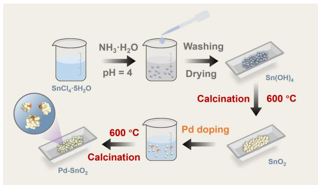
**Figure 4.** Schematic diagram of the formation of Pd-doped  $\text{SnO}_2$  MEMS gas sensor.
