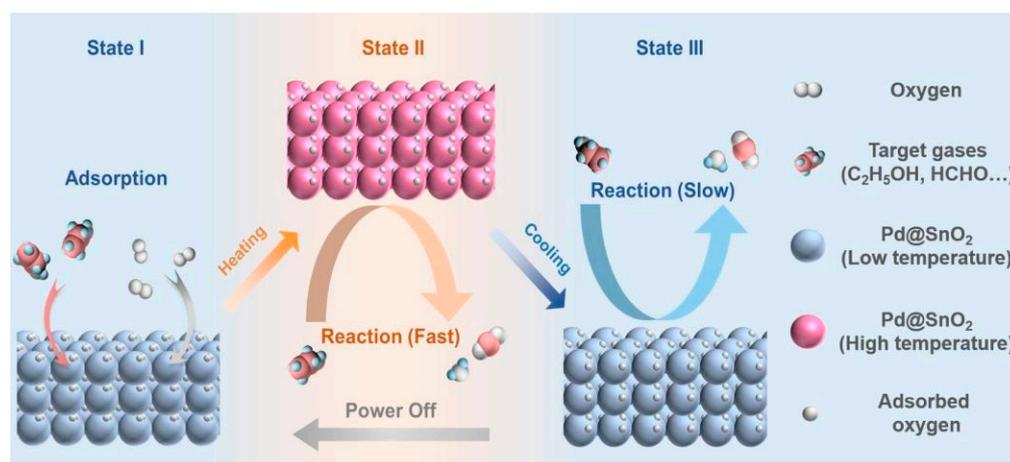
**Figure 8.** Schematic diagram of sensing mechanism of the MHP gas sensors under PWM excitation method.
