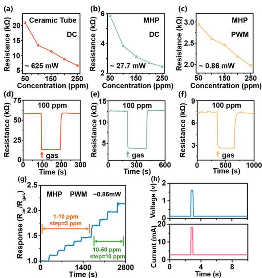
**Figure 7.** Operating resistance curve under (a) DC heating on ceramic substrate (b) DC heating on MHP and (c) PWM heating on MHP. (d–f) Response–recovery curve on exposure to 100 ppm ethanol. (g) Response to 0–50 ppm ethanol at 1 mW. (h) Measured voltage and current value for power consumption.
