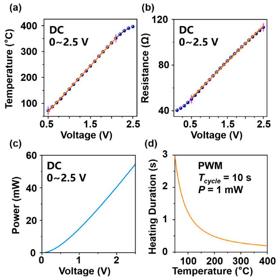
**Figure 3.** (a) The temperature variation in the MHP with applied DC voltage (b) The resistance of the micro-heater under different applied DC voltages (c) The power consumption of the micro-heater under different applied DC voltages (d) The maximum heating duration ( $T_{on}$ ) when  $T_{cycle} = 10$  s,  $p = 1$  mW.
