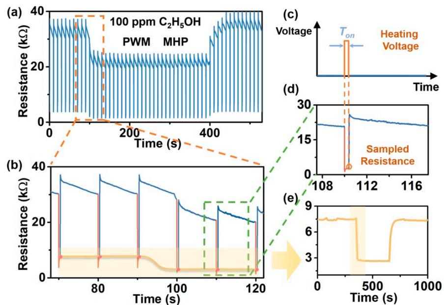
**Figure 6.** Resistance sampling under PWM excitation method. (a) Detailed resistance value of the response–recovery curve on exposure to 100 ppm ethanol. (b) Enlarged view of the response stage on ethanol vapor. (c) Heating voltage in one cycle under PWM excitation method. (d) Detailed resistance value under single heating cycle. (e) Response–recovery curve on exposure to 100 ppm ethanol.
