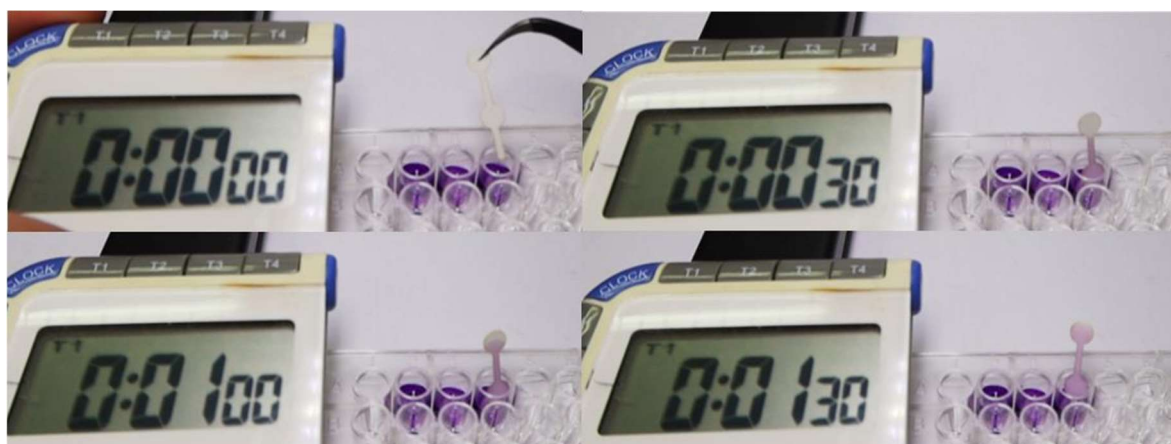
Figure S9. Time required for an aqueous solution containing crystal violet dye to move through the dipstick.
